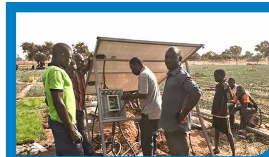
ICBA set up solar-powered irrigation systems in Burkina Faso and Mali for more than 100 smallholders. The system saves about 40 percent of irrigation water compared with traditional surface irrigation systems.
